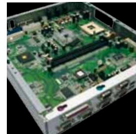
Motherboard in steel housing
